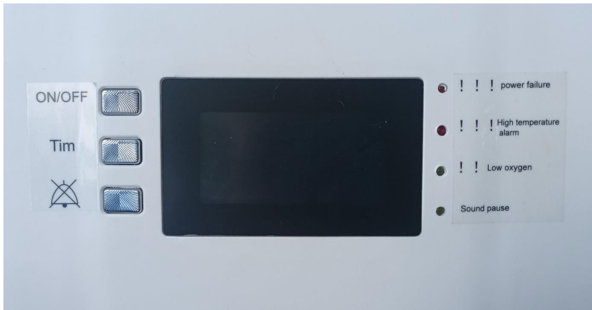
Oxygen concentrator control panel, showing on/off control, timer control and alarms.
